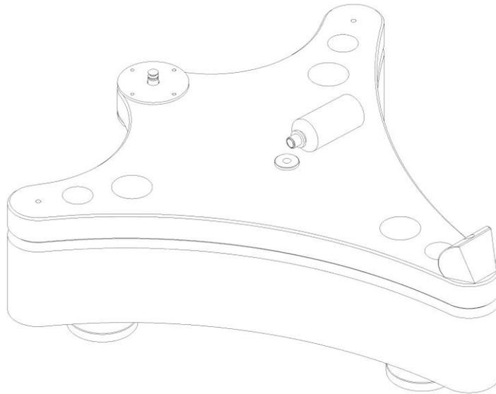
Installing the platter.
