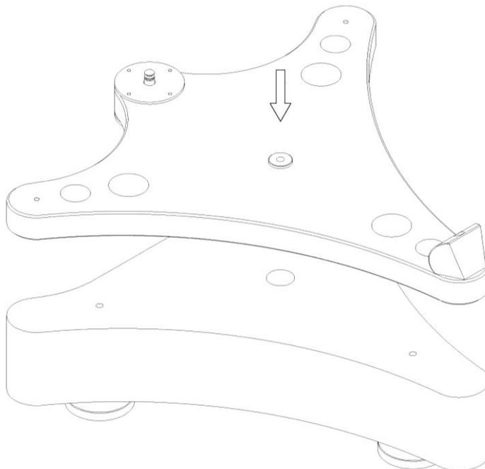
Fill the bearing with lubrication oil supplied to a level of approx 1mm above the bottom bearing.
