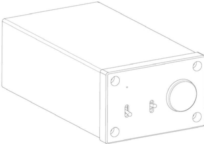
The knob on the right side of the speed controller is for adjusting the speed by speed strobe.
