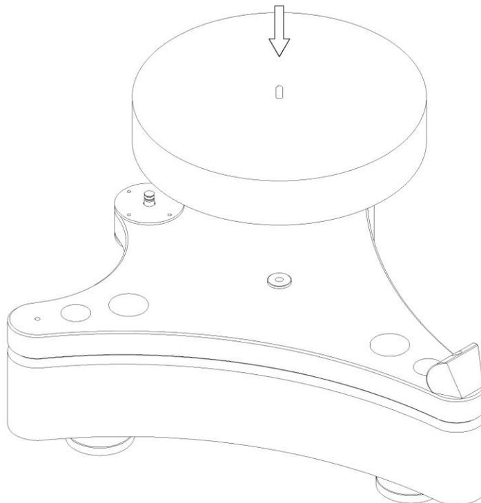
Take out one of the drive 'belts' and run it round the motor spindle and then round the platter.
